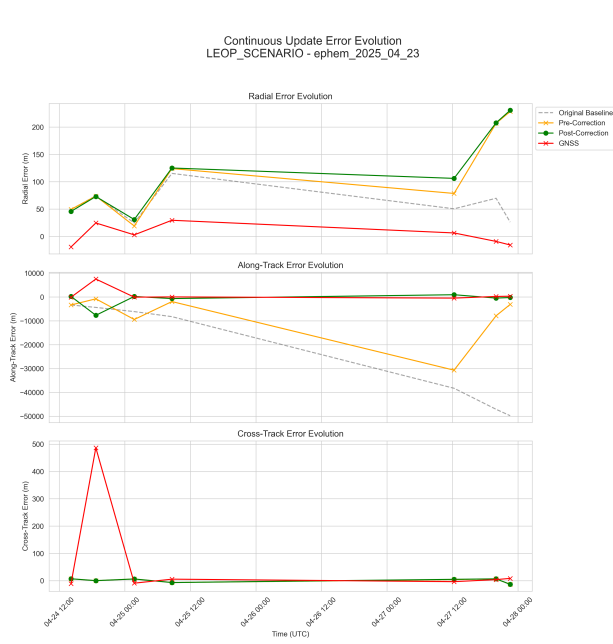
Fig. 5: Baseline, pre- and post-correction, and GNSS errors at each track update during the LEOP simulation scenario for Sat. B.
