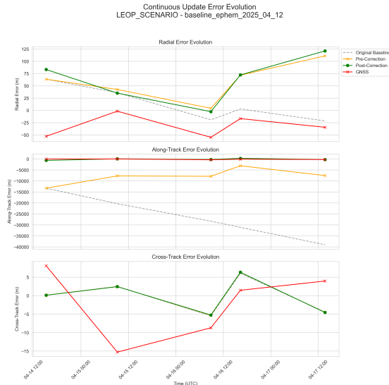
Fig. 2: Baseline, pre- and post-correction, and GNSS errors at each track update during the LEOP simulation scenario for Sat. A.
